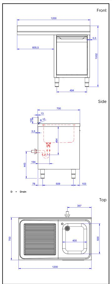
Drain: **Drainer position:** Left **Key Information:** Cabinet width: 1145 mm Cabinet depth: 645 mm Cabinet height: 385 mm 1200 mm External dimensions, Width: External dimensions, Depth: 700 mm External dimensions, Height: 1000 mm **Upstand Dimensions, Height:** 100 mm Upstand Dimensions, Depth: 13 mm Upstand Dimensions, Radius: R=10 **Bowls number Bowl dimensions** 400x500xH300 Number and type of doors: 1 Hinged Worktop thickness: 50 mm Net weight: 55 kg
